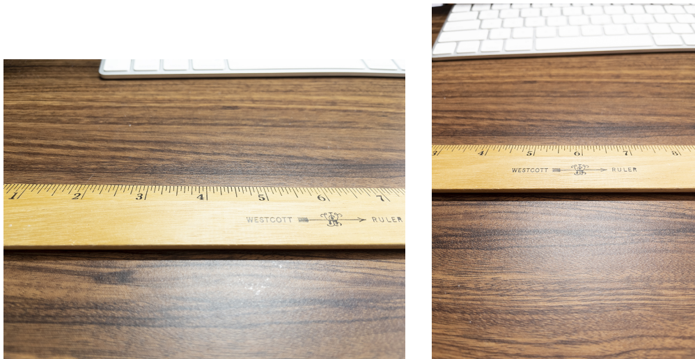
Figure 8: Finding the field-of-view of a camera/lens combination
